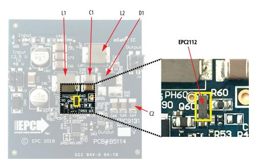
Figure 3. Photo of EPC9131 SEPIC regulator with EPC2112.
