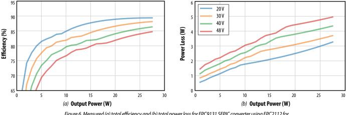
Figure 6. Measured (a) total efficiency and (b) total power loss for EPC9131 SEPIC converter using EPC2112 for various input voltages delivering 19 V output over the load range from 1 W through 27 W.
