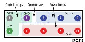
Figure 4. Bump assignment for easy layout.
