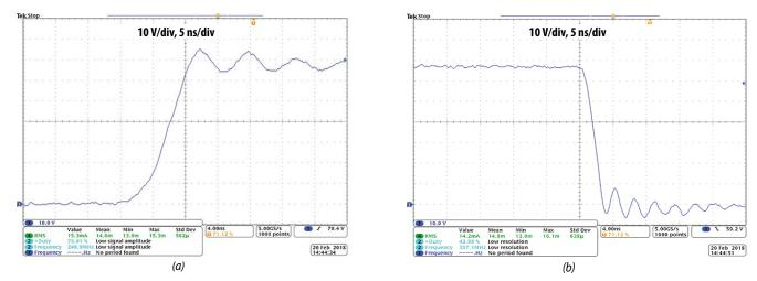
Figure 7. Switch-node voltage waveforms of the SEPIC at 48 V input, 19 V and 27 W output. (a) rising edge and (b) falling edge.
