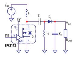
Figure 2. Schematic of SEPIC using EPC2112 with integrated gate driver.
